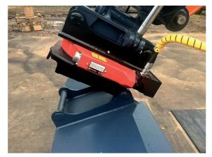
Attaching the tool to the rotator.
