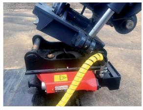
Removing the rotator from the connector.
