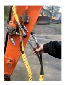
Connection of hoses to boom hydraulics.
