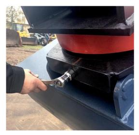
Tool locking screw to the OPEN position.
