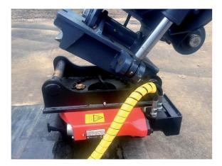
Mounting the connector on the rotator.
