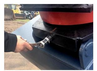
Tool locking screw to the CLOSED position.
