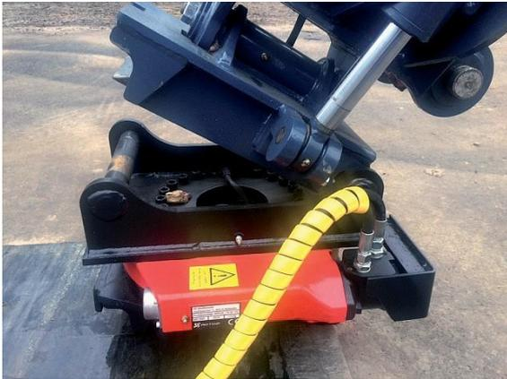
*Removing the rotator from the connector.*
