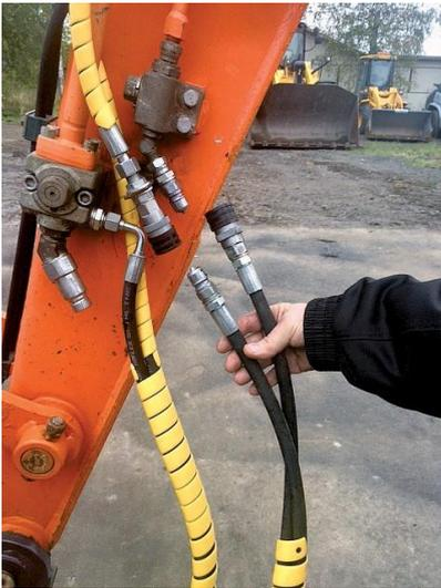
*Connection of hoses to boom hydraulics.*
