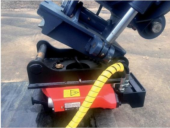
*Mounting the connector on the rotator.*
