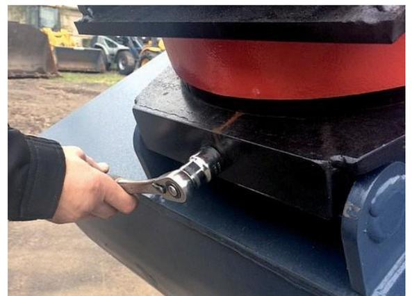
*Tool locking screw to the CLOSED position.*
