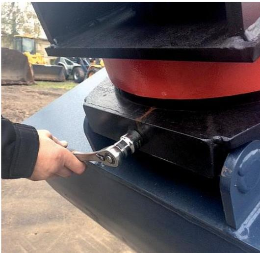
*Tool locking screw to the OPEN position.*
