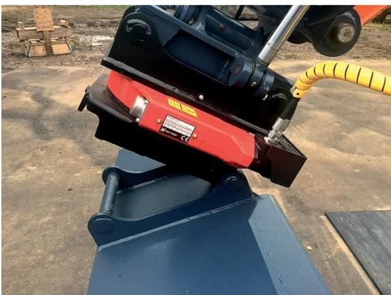
*Attaching the tool to the rotator.*
